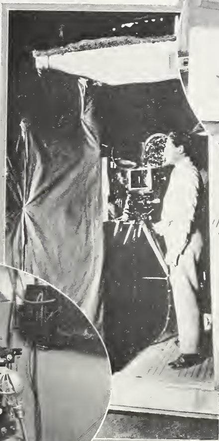
Center: Taking the Picture in a Sound Proof Booth; Left: Recording the Sound on a Wax Disk; Above: the Synchronized Projection of Film in the Projector and of Sound from the Disk in a Theatre Projection Booth
